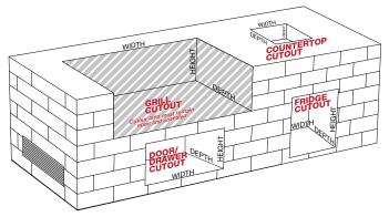
All stated dimensions below are accurate but as tape measures and grill bodies can vary by  $\frac{1}{6}$ ", we recommend measuring and confirming your purchased unit before installing or constructing your barbecue island.
